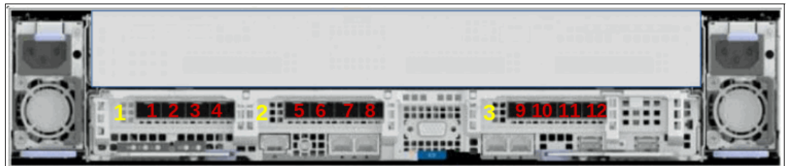
Figure 2-9 Port location in FlashSystem 9100 rear view
